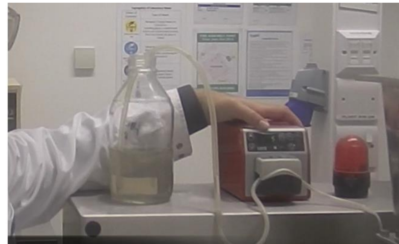
The binder feed rate is selected. The operation conditions are checked to provide a continuous feed.
