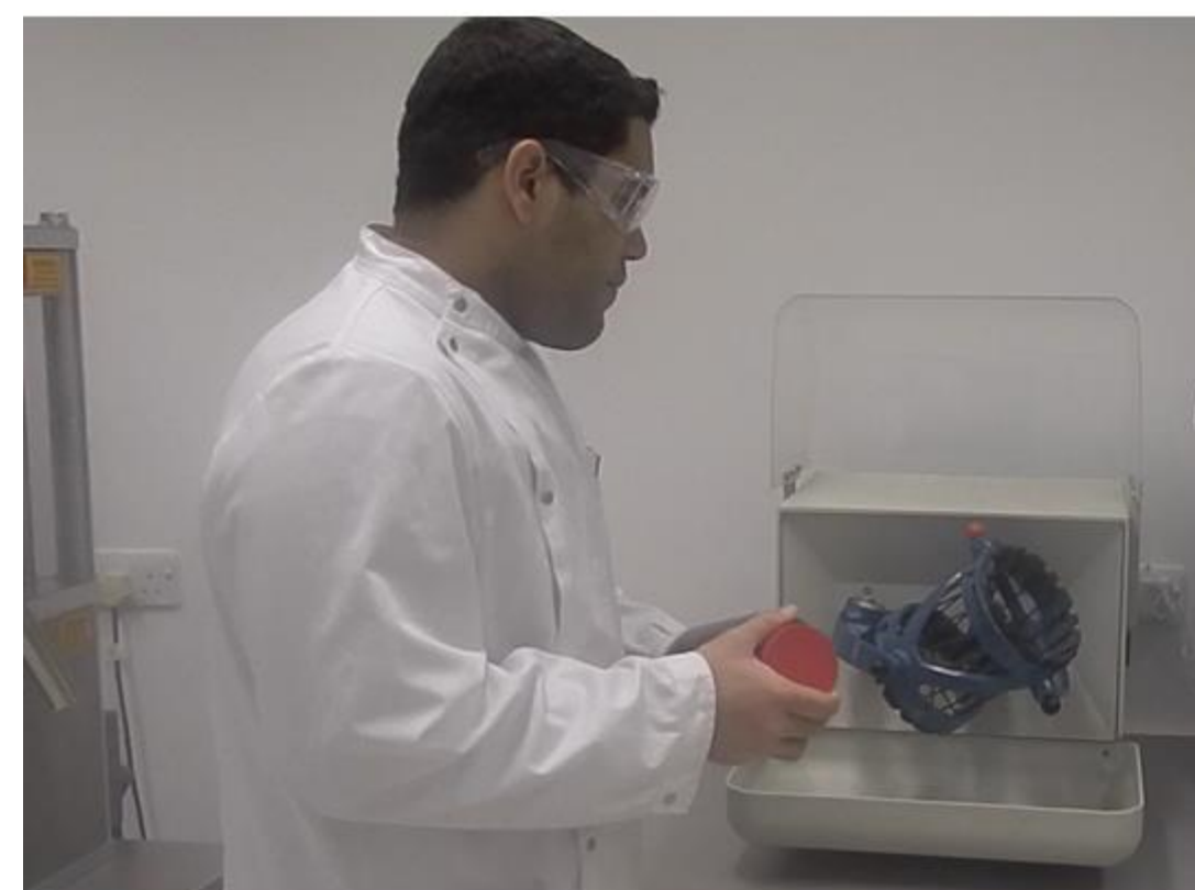
The formulation is mixed in a Tubula shaker mixer
