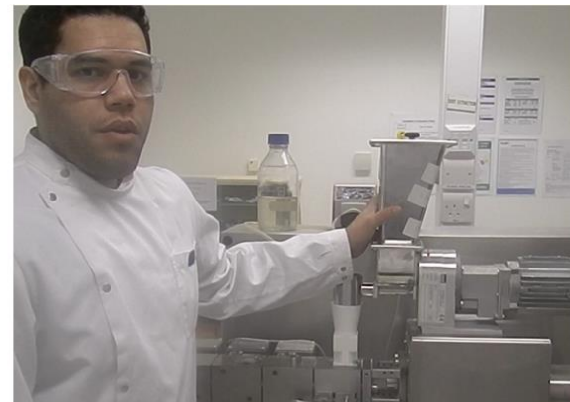
Twin screw solid feeder is kept between 30-70% of full capacity. Feed rate is set to desired throughput
